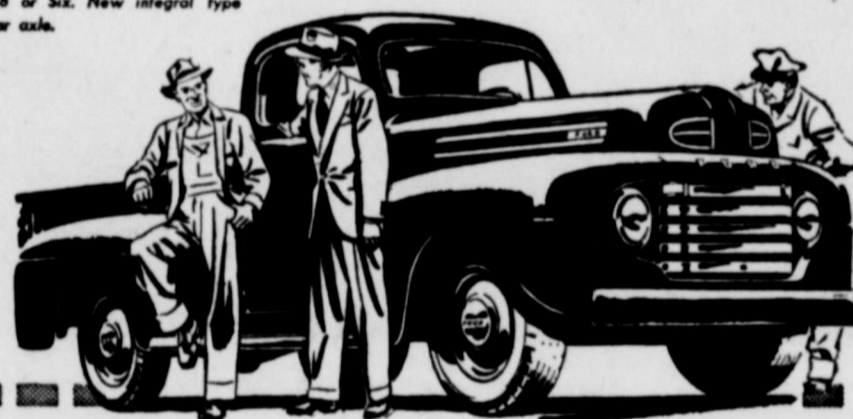
Ford 6 1/2 ft. half-ton Pickup. G.V.W. 4,700 lbs. Choice of two engines, V-8 or Six. New integral type rear axle.
