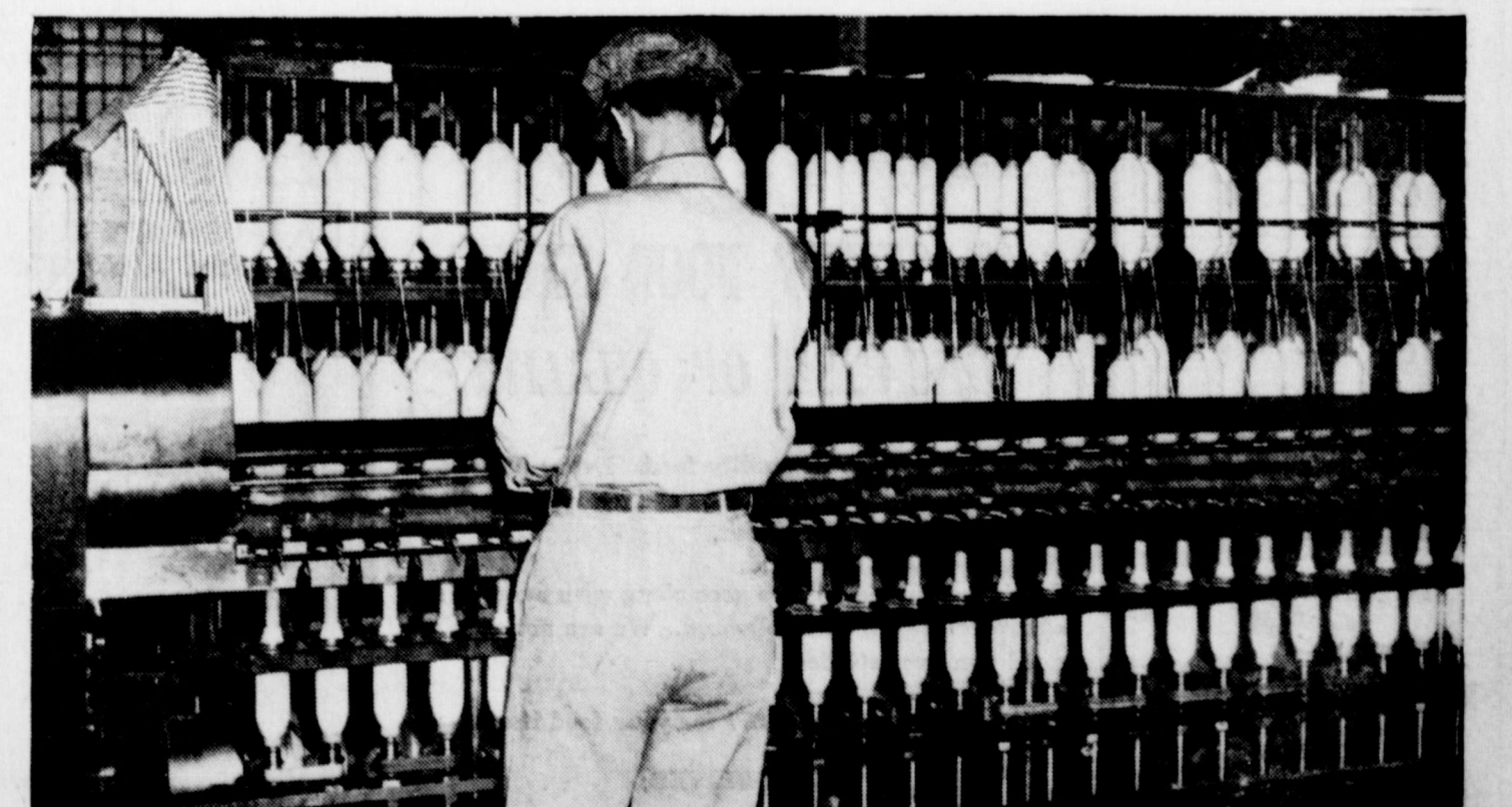
INMATE OPERATES A ROW OF SPINNING MACHINES. OPERATION REDUCES YARN, SPINS IT ON SPOOLS.
