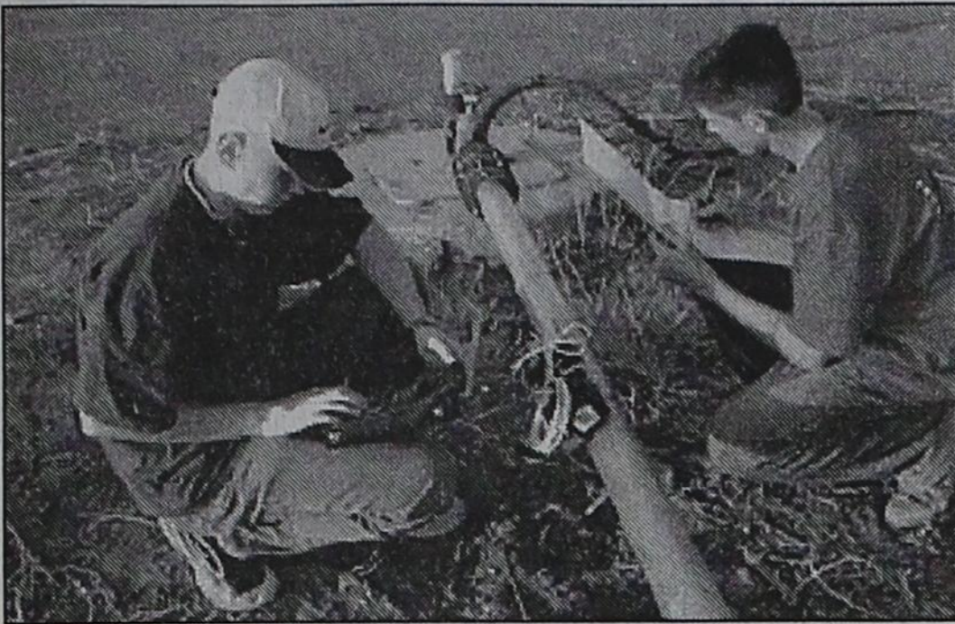
Matthew White (left) and Pat Hunter (right) checking irrigation well with Panametric Flow Meter ...
