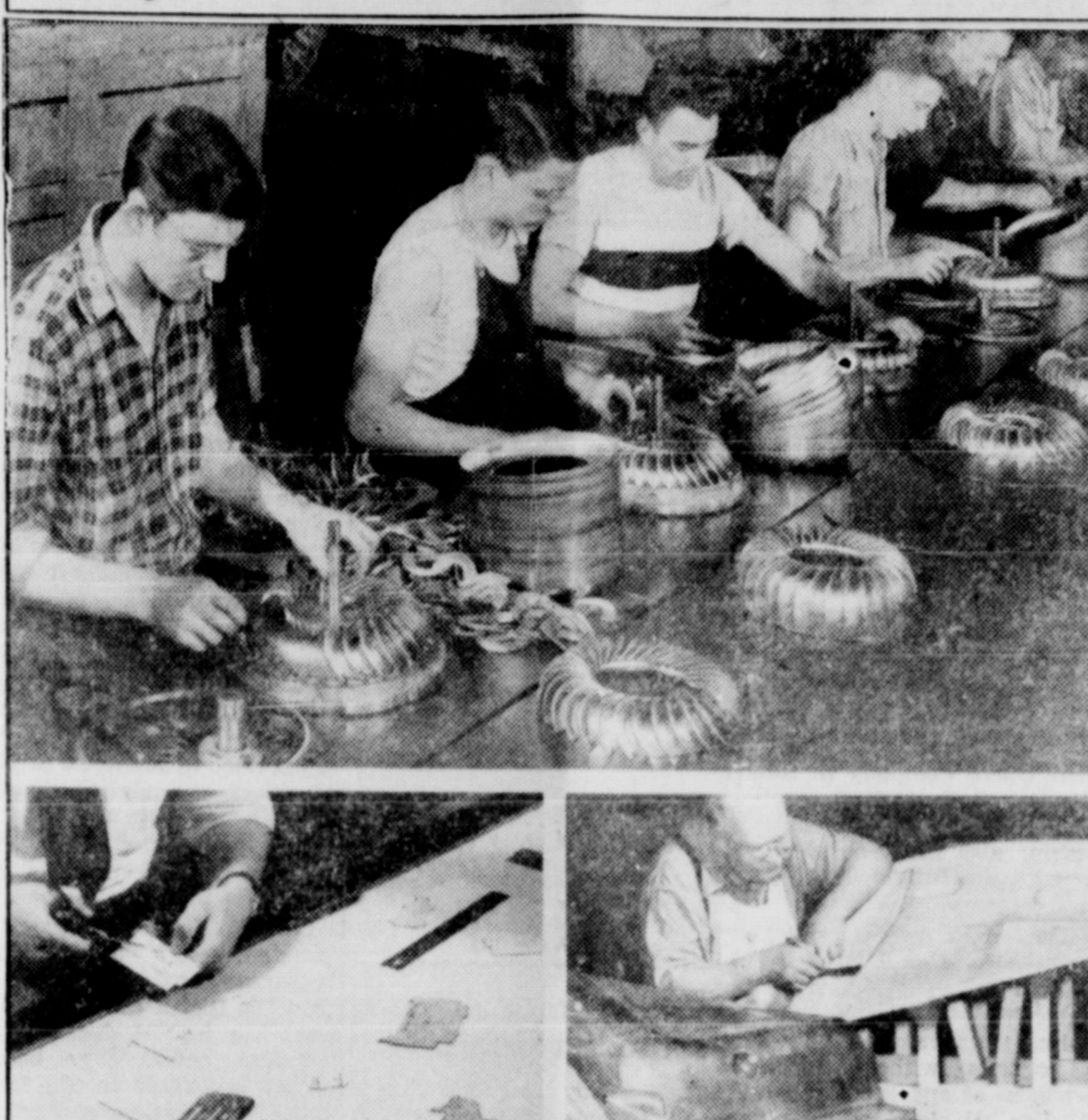
Skillful hands continue in demand in the manufacture of automobiles, despite the rise of machines. Here's evidence in pictures taken at the Chevrolet plant: (Top)—A crew positions 60 vanes of the Powerglide automatic transmission before the assembly is spot welded. (Lower left)—To plan factory layouts draftsmen cut out cross-sections of the floor area of machines at scales of precisely one-quarter inch to one foot. (Lower right)—A pattern-maker builds a wooden model that will later be duplicated in steel to stamp out thousands of fender parts.
