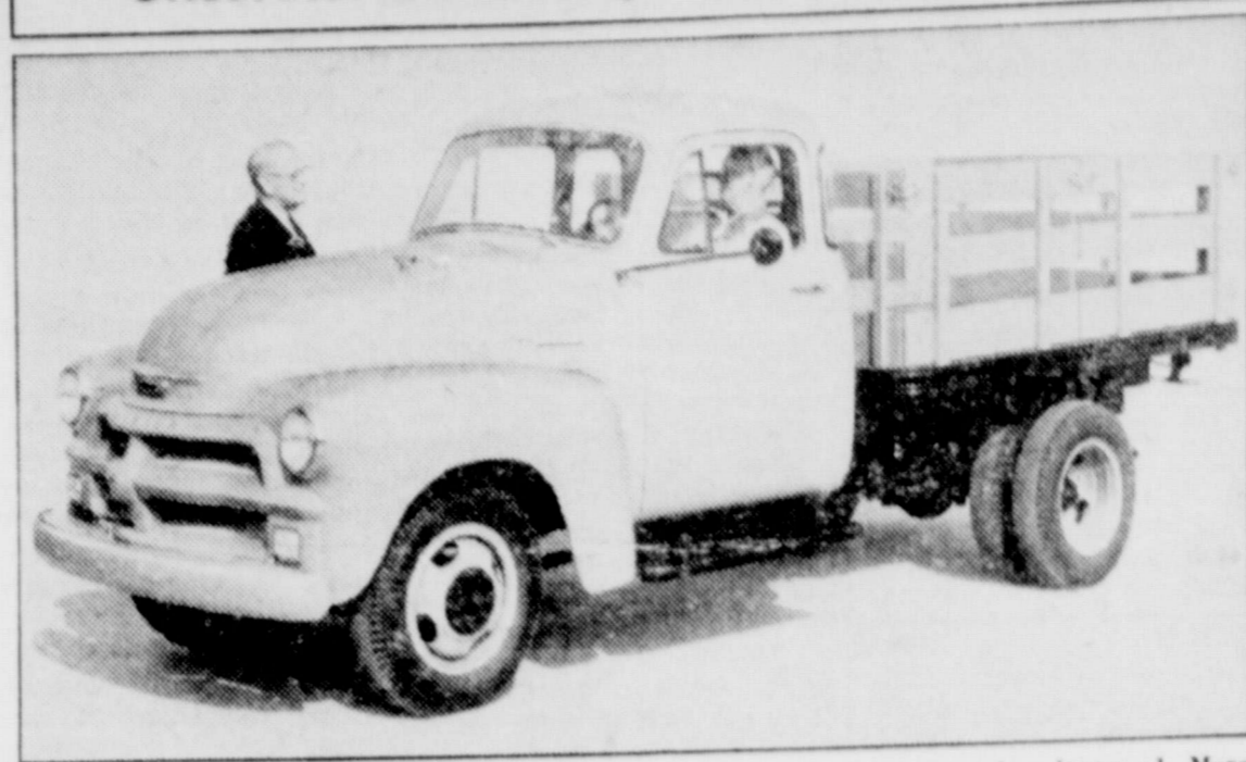
Typical of completely re-engineered Chevrolet trucks making their 1954 model debut at dealer showrooms this week is the three-quarter ton (6500 GVW) stake, on which dual rear wheels are now available. Loading height has been lowered and floor area between stakes increased. More horsepower in each of three new engines, greater durability through sturdier construction, optional automatic transmission, improved comfort and convenience are among Chevrolet truck advances.
