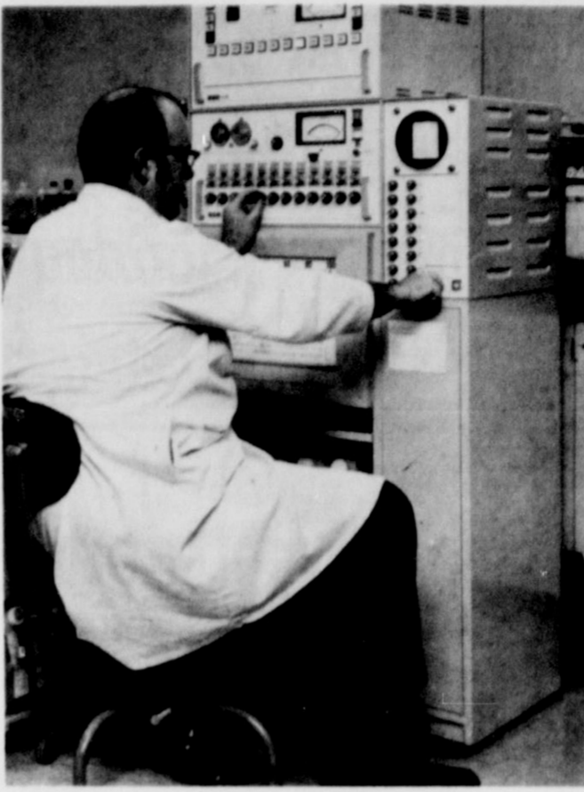
EQUIPMENT AT HI-PLAINS. Richard Lanier, lab technician at Hi-Plains Baptist Hospital, is shown operating the new SMA 12/60 machine which produces 12 different chemical tests at one minute intervals.
