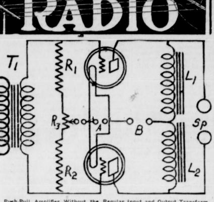
Push-Pull Amplifier Without the Regular Input and Output Transformers. A Potentiometer is Used to Divide the Secondary Voltage of Transformer Between the Two Tubes. Two Choke Coils Are Used in the Output and the Loudspeaker is Connected Directly Across the Coils Without Any Stopping Condensers.
