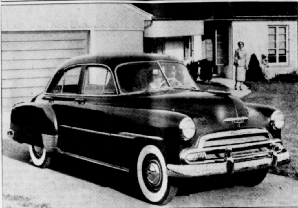
The Styleline De Luxe four-door sedan is one of 14 models introduced by Chevrolet as its passenger car line for 1951. Notable in this picture are the design improvements which accentuate a longer, lower appearance. Radiator grilles have been simplified, the decorative body moulding lowered and rear fender crowns raised. Models also offer added safety.
