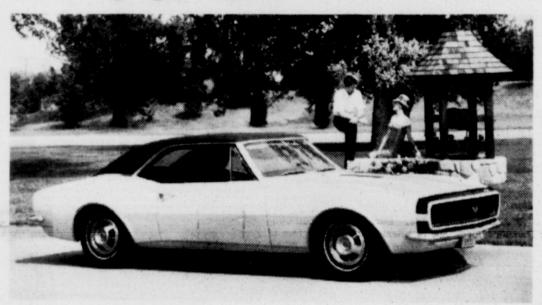
The all new CAMARO will be built in sport coupe and convertible models (Super Sport shown above). The Camaro line incorporates many sprightly options that include concealed headlamps behind a lattice grille which opens and closes when lights are turned on and off, plus a hood with simulated louvers and a wide "bumble bee" paint band on the nose. A 350-cu.-inch V8 engine is used in the Super Sport version of the CAMARO. They go on display September 29.
