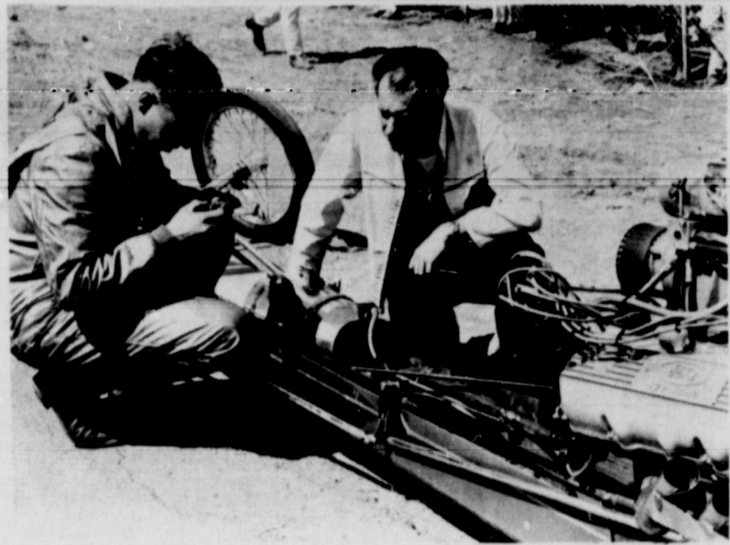
READY FOR ACTION... Kalitta, left, examines fuel line jet that feeds this 1400 H.P. Ford engine. This is "The Bounty Hunter", one of the exotic cars that AA fueler drivers use to attain money, fame and glory. "The Bounty Hunter" piloted by Kalitta is just fresh from winning the winner Nationals Championship in Pomona, California. Kalitta blasted through the quarter mile at the unbelievable speed of 219.50 miles per hour with an elapsed time of 7.17 seconds. Kalitta will be featured on the season opening program this Sunday at the Amarillo Dragway, 7 miles south on Washington in Amarillo, Texas, as he pairs off in open competition against over sixteen of Amarillo Dragway's regular runners who put down two National Champions in 1966. The action is slated to get underway this Sunday afternoon at 2:00 p.m.
