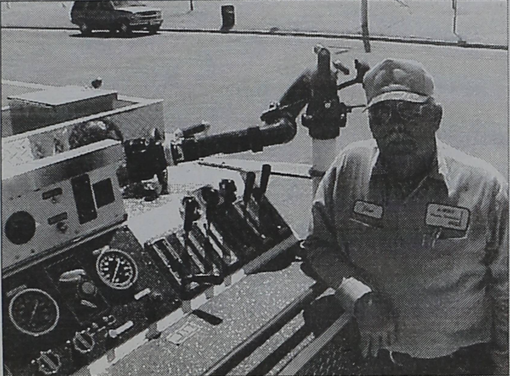
CONTROL PANEL... Fire Chief Jim Taylor is shown at the controls of the city's new fire truck. The pump nozzle over his right shoulder is capable of pumping 1000 gallons of water in one minute. ron carr photo
