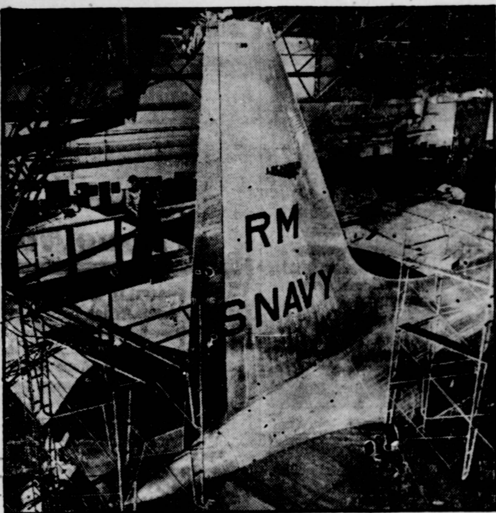
TALL TAIL TEST —Fifty feet above the floor of a hangar at Ames Aeronautical Laboratory, Moffett Field, Calif., technicians install pressure measuring equipment in the towering tail of the Navy's Lockheed Constitution transport plane. Research flights will provide valuable data on tail loads during flight of very large aircraft. The Constitution, with a wingspan of 189 feet, will have a maximum weight of approximately 80 tons during the tests.
