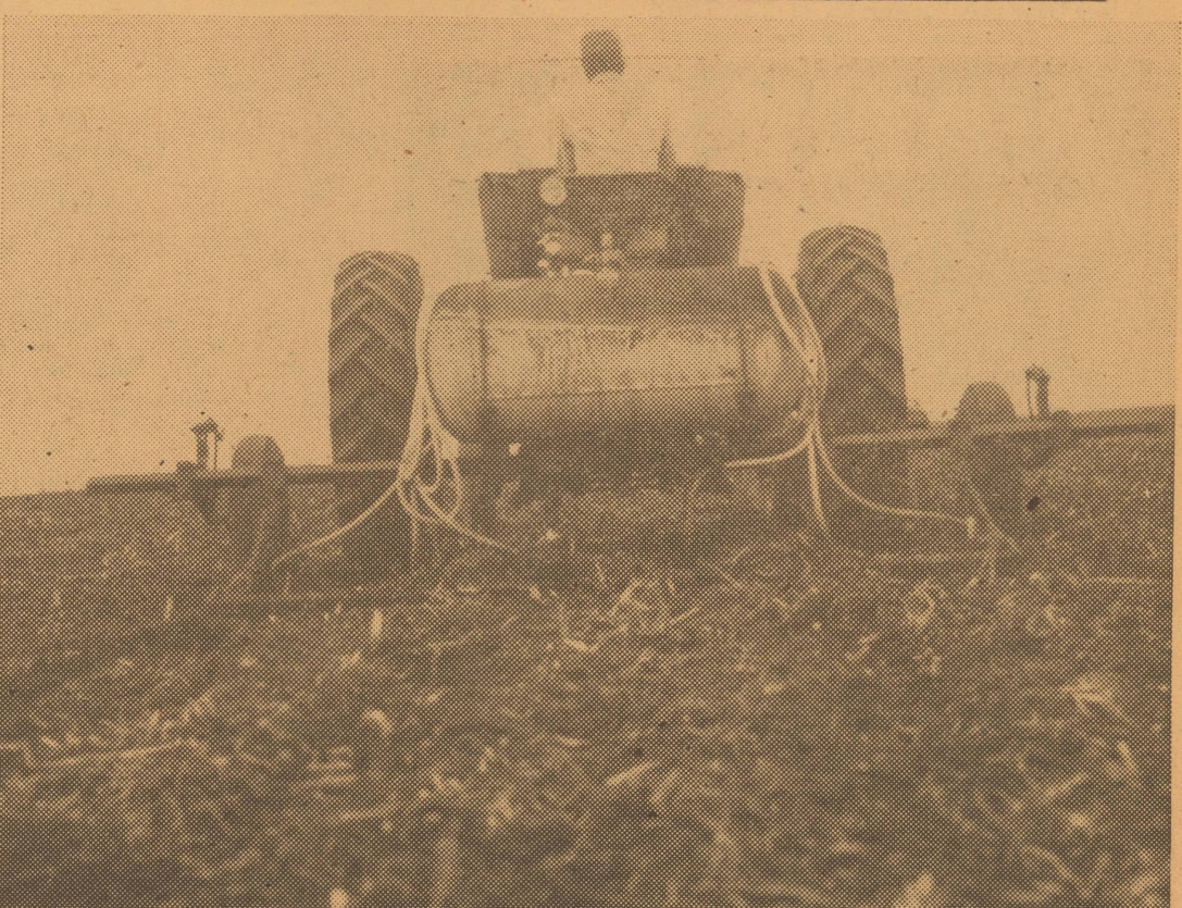
Some farmers are still putting ammonia-type fertilizer on their grain sorghum stubble. Tractor-mounted rigs such as this one are very popular. Many farmers put on their own fertilizer in this manner, renting the rigs and purchasing the fertilizer from dealers.
