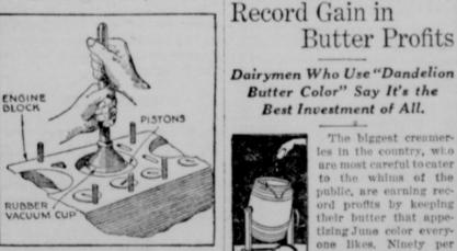
Testing for Loose Wrist Pin or Con. necting Rod Bearing With a Plumber's Force Pump.
