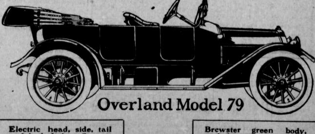
and dash lights; Storage battery; 35 H. P. motor; 114-inch wheelbase; Tim-ken bearings; Splitdorf magneto; Model R Schebler carburetor: Threequarter floating rear axle; 33x4 Q. D. tires; Cowl dash.
