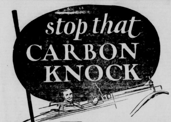
CARBON KNOCK or motor detonation aside from being annoving greatly reduces power efficiencycombustion taking place before the complete rise of the piston. The mechanical method of correcting such knocks is to retard the spark which again reduces power efficiency.
