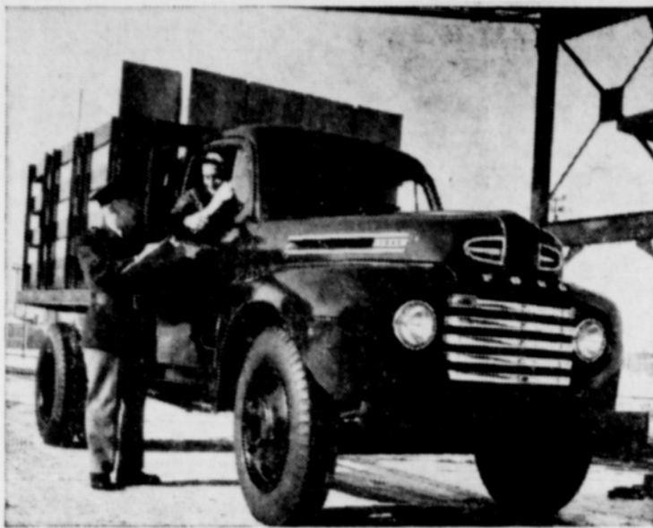
The new 1948 series F-5 Ford 1 1/2-ton, 134-inch wheelbase truck with a nine-foot stake body was shown to the public today by the Ford Motor Company. The new truck line represents the first postwar products of Ford and is offered in a wider range of models and capacities than ever before, from 1/2-ton pick-up and panel models through 2 1/2- and 3-ton series F-7 and F-8, the largest trucks the company has ever built.
