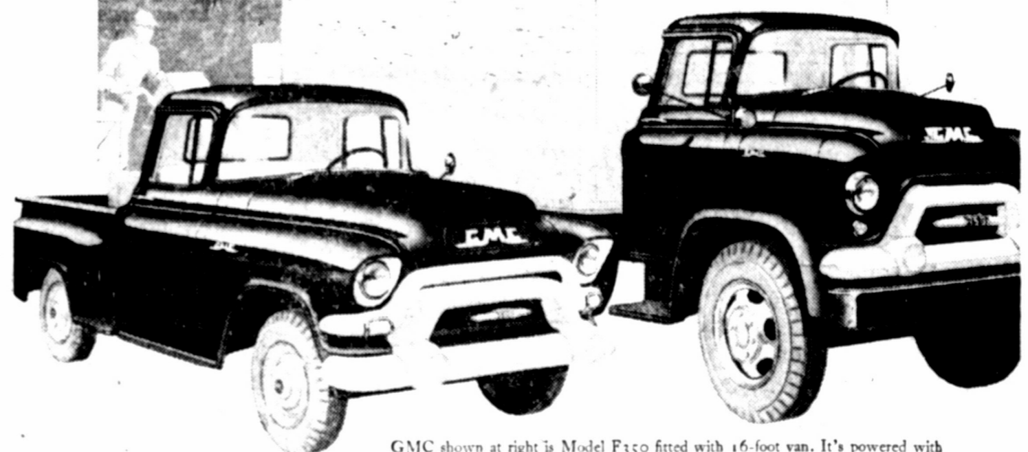
GMC shown at right is Model F350 fitted with 16-foot van. It's powered with a 140 h. p. six-cylinder engine—has over-size axles rated at 4,500 lbs. front; 14,000 lbs. rear. It's designed for 18,000 GVW truck-work. The smaller truck at left is GMC's popular 1/2-ton pickup with a 130 h. p. six-cylinder power plant.
