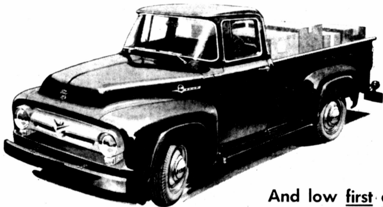
Ford's F-100 pickup with 8-ft. box is the biggest in the half-ton field—up to 19 cu. ft. more loadspace than the others. Regular 6 1/2-ft. box with a full 45 cu. ft. capacity also available.
