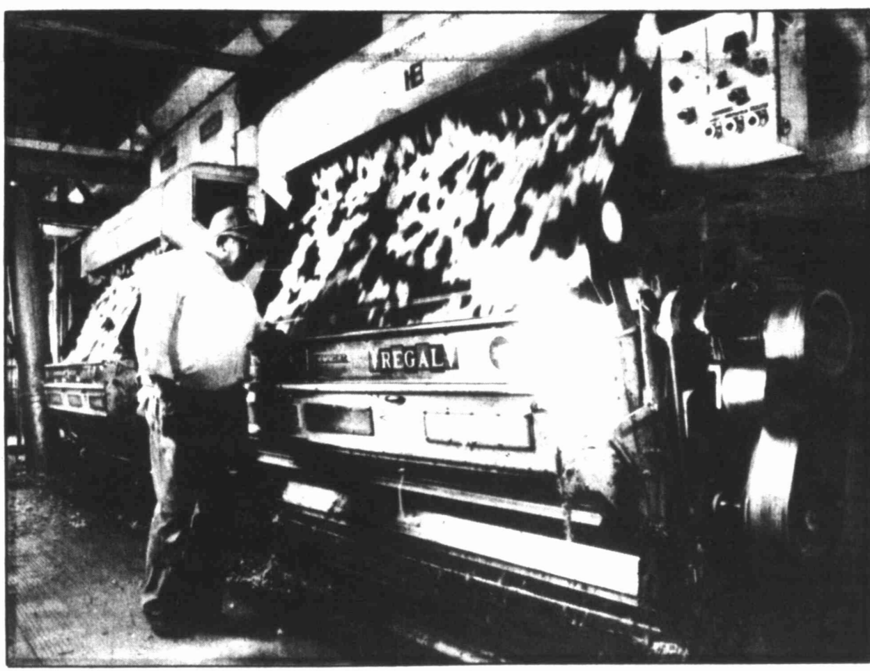
Area ginners run their operations day and night to keep up with the high volume of cotton that comes in during cotton ginning season. In the pictured process, any exterior matter surrounding the cot-
