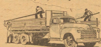
Heavy-Duty Long Wheelbase with Trailing Axle
