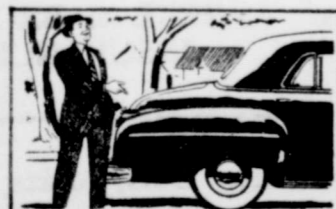
FENDERS are bolted on . . . easy on your pocketbook to repair, or even replace, if dented or damaged.
