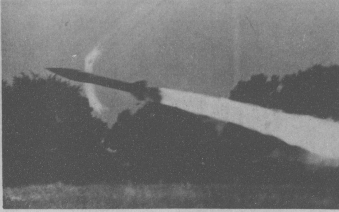
"DON'T BLINK OR YOU'LL MISS IT"-- An Honest John rocket streaks from its launch carrier at the Sept. 13 demonstration firing by Battery A, 1st Battalion, 16th Artillery, 2nd Armored Division. About 250 civilians and military personnel witnessed the event, which indeed happened so fast that a blink would have obscured it completely. The flames coming from the sides of the projectile are "spin rockets," which impart stability to its flight.
