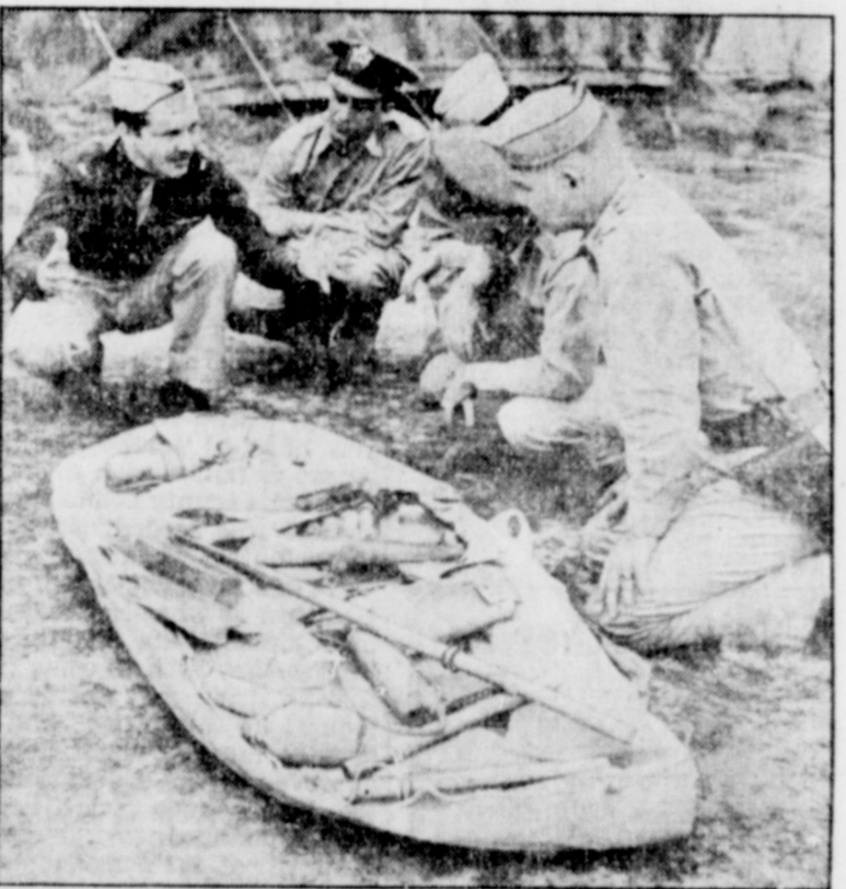
Flyers at Hawaii learn important lessons in the use of collapsible life-rafts, because most of their flying is done over water. Each raft is equipped with gas-bottle inflater, flares, oars, rations, water, pump, first-aid kit and rubber patching kit.
