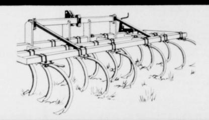
CHISEL PLOW . . . versatility with extra trash clearance, rigid clamps and swedge-point
