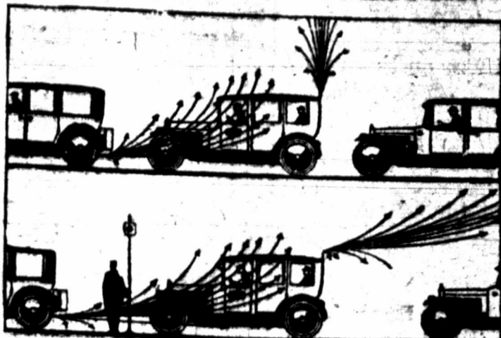
New carbon monoxide fumes from horizontal exhaust affect the driver behind and how the vertical exhaust avoids this; above at a standstill, below in motion.
