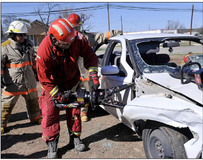
Alan Garner of Advanced Rescue Systems demonstrates how to use a battery powered "Jaws of Life" spreader during Saturday morning's training at the Sonora Fire Department.
