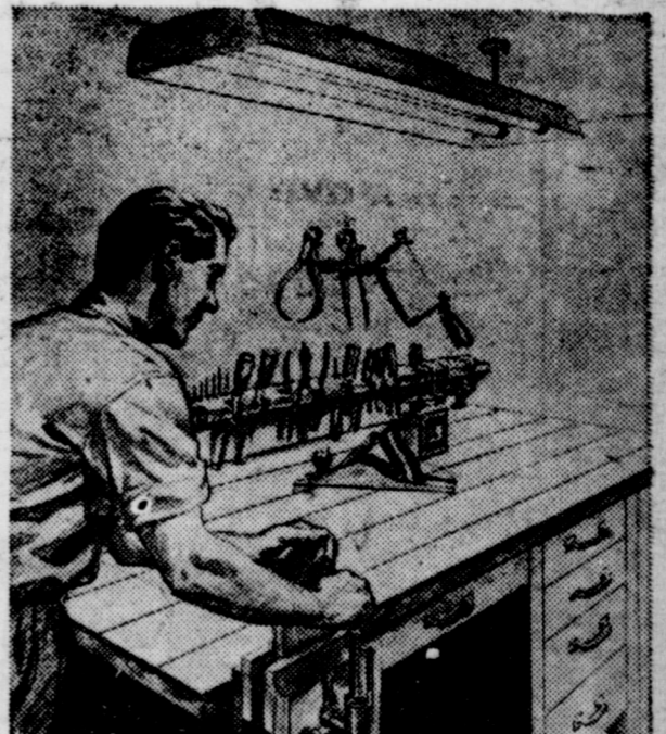
For working at bench with a ceiling light, this fixture—holding two 25-watt fluorescent tubes, shielded lengthwise—will give you an excellent light. Or you can use a 150-watt silver-bowled bulb in a round metal reflector 12 to 14 inches in diameter.
