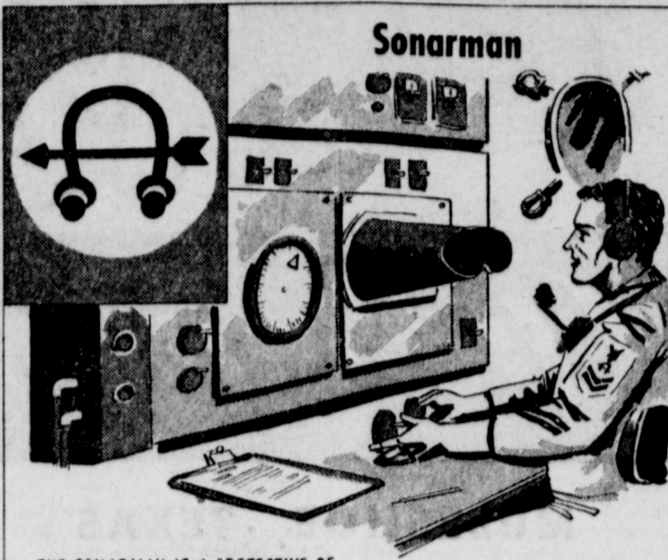
THE SONARMAN IS A "DETECTIVE OF THE DEEP." HIS ELECTRONIC SOUND EQUIPMENT IS ABLE TO DETERMINE WHAT IS UNDER THE WATER; TO DETECT UNCHARTED REEFS, ENEMY SUBMARINES OR OTHER SUBMERGED OBJECTS. OPERATION AND CARE OF SENSITIVE SONAR EQUIPMENT IS THE SONARMAN'S DUTY. THE OIL WELL SOUNDING DEVICE OPERATOR IS THE CIVILIAN COUNTERPART OF A SONARMAN.
