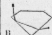
B TOO THICK "Leaks" light and has "sleepy" cost
