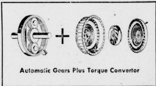
Automatic Gears Plus Torque Converter
