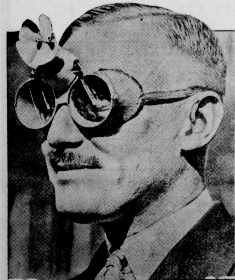
This is L. A. V. Davoren of England wearing a pair of the "rain goggles" that he has invented. They are fitted with windscreen wipers which are driven by an exterior air fan that comes into operation when the motorist is traveling at a speed of fifteen miles an hour or upwards.
