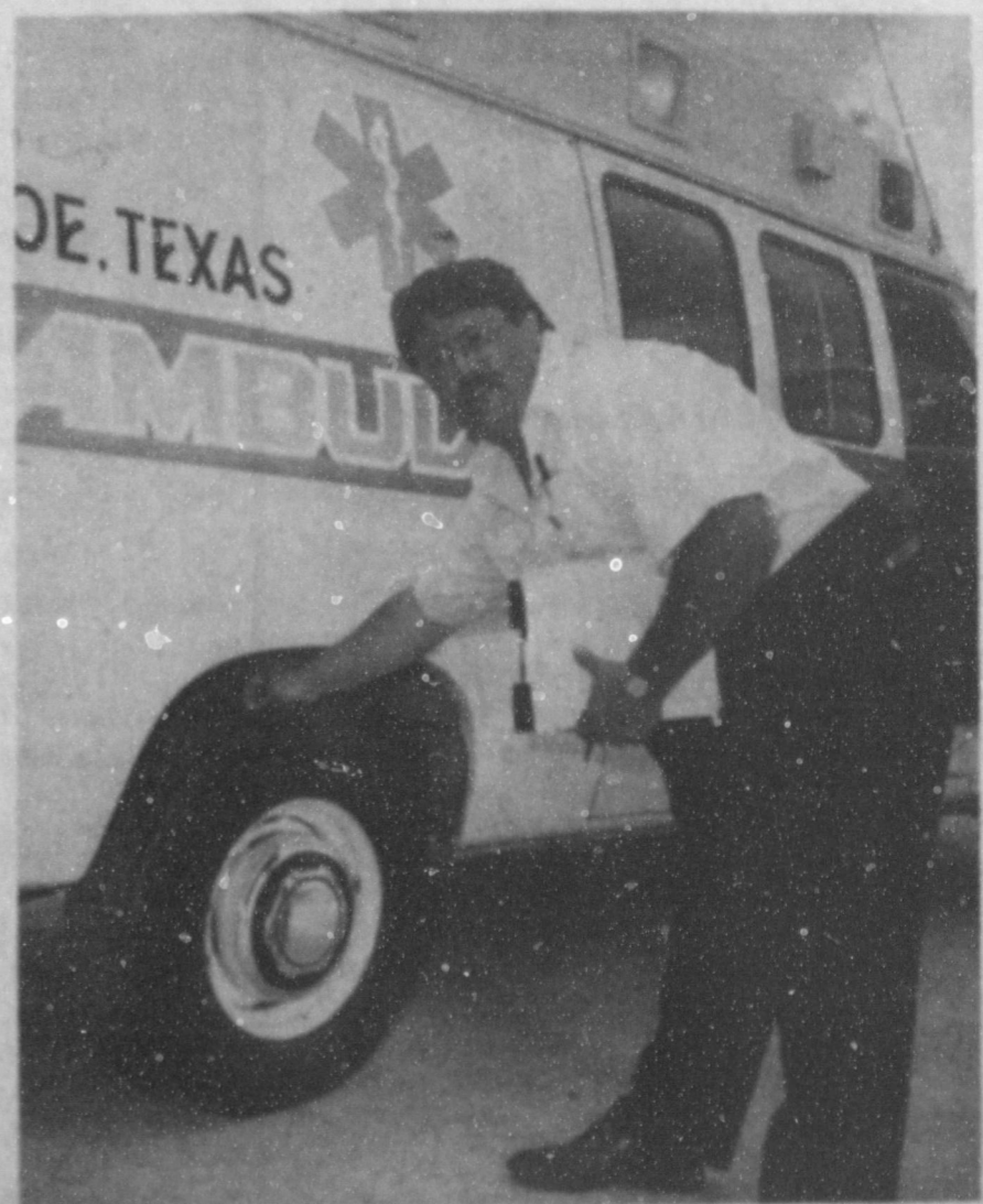
AMBULANCE INSPECTIONS HELD--Denny Martin, EMS Field Consultant for the Texas Department of Health, was in Muleshoe Monday to inspect Bailey County Ambulance Service's two ambulances. Here, he is shown measuring the depth of tread left on a tire. He re-certified the ambulances, but recommended new tires for the ambulances. (Journal Photo)
