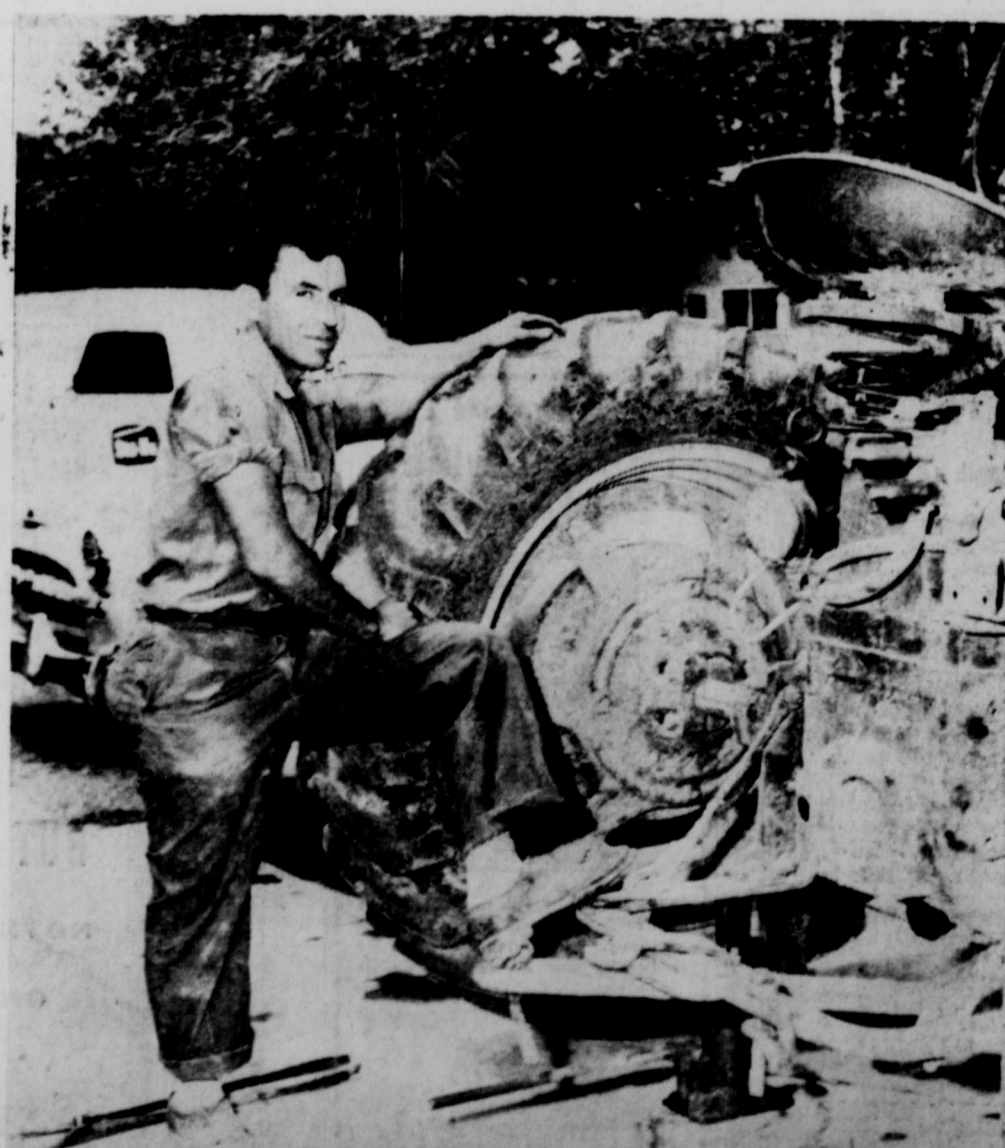
MANUEL SOSA prepares to dismount a huge tractor tire which will be repaired or recapped by Pior Rubber Company. Pior's is equipped to go into a farmer's field, remove the weighting chemicals, repair the tire, and replace the chemicals. The company is equipped with the most up-to-date tools and machinery.
