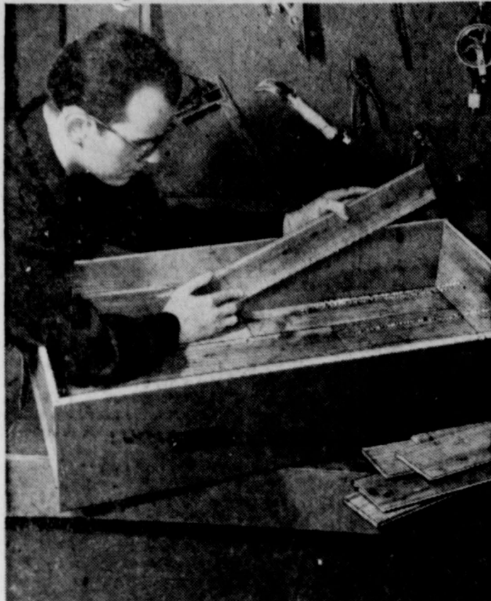
Moth-proof dresser drawers by lining them with aromatic red cedar closet lining. The fragrant cedar aroma keeps moths away from woollens and other items stored in the drawers. Readily available tongued and grooved pieces of cedar make the job an easy one.
