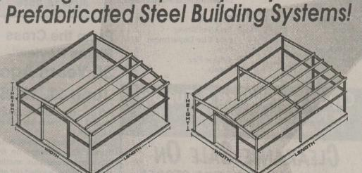
· NO WELDING REQUIRED · CLIPS WELDED IN PLACE FOUNDATION & ANCHOR BOLT DRAWINGS MARKED FRAME COMPONENTS SHORT LEAD TIME • ERECTION DRAWINGS
