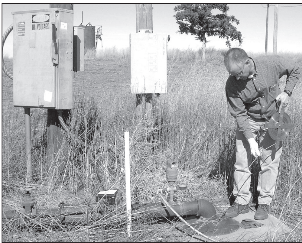
Keith Whitworth making a depth-to-water level measurement in an observation well near Whiteface in Cochran County.
