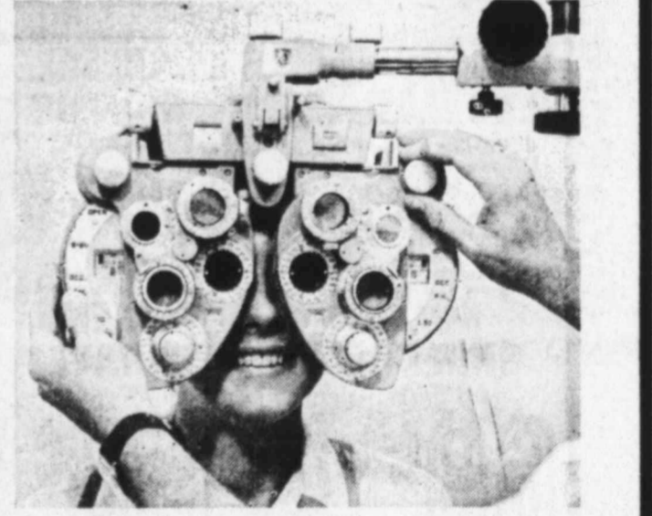
The phoropter is used to determine the corrective prescription required, if any.
