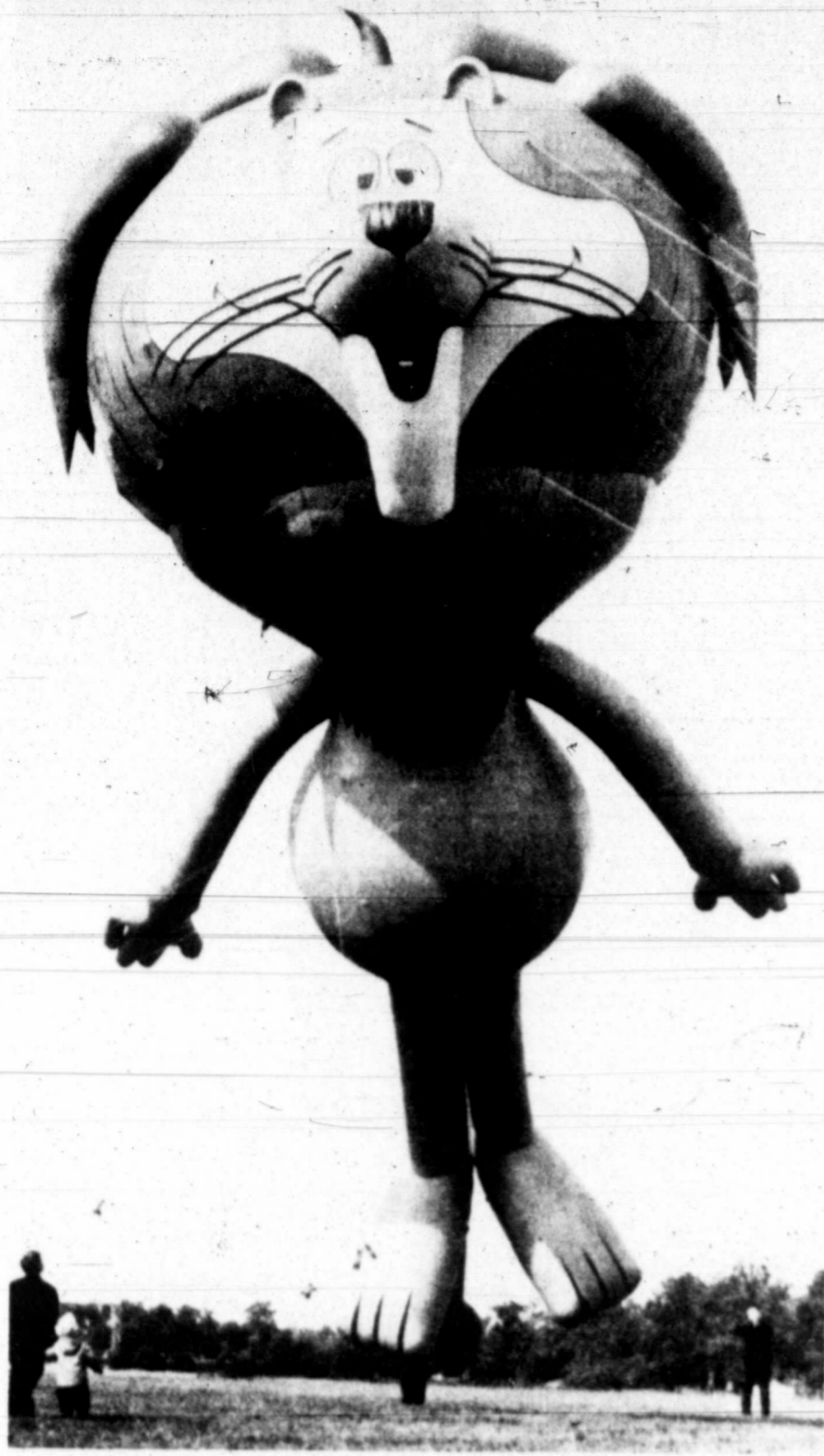
Linus, a 55-foot-tall figure balloon created by Goodyear Aerospace Corporation for Macy's Thanksgiving Day Parade is kept aloft by 7,500 cubic feet of helium and requires more than 40 handlers to hold him down. (AP Laserphoto)
