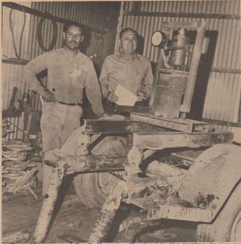
Pete Almaguer and Pat Ballew standing beside the testing device to test oil field anchors, mobile home anchors and high line anchors for the new company, Seminole Mobile Home Anchor, Inc.
