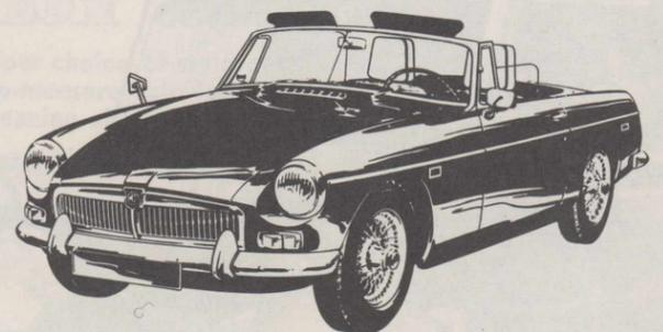
For performance: a 1798 c.c. twin-carb engine, fully synchronized four-speed gearbox, heavy-duty suspension, rack-and-pinion steering, and dual braking system with disc brakes up front.
