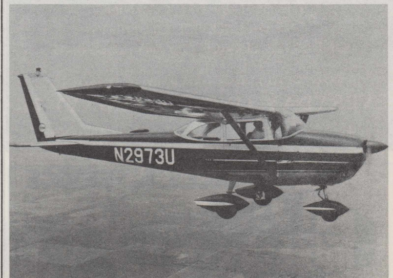
NEW TRAINER — This Cessna 172 propeller-driven plane will be used to start Reese pilot training in about a year. It has been purchased by the Air Force for use of civilian contractors in the first 30 hours of Reese training. The 172 has a top speed of 138 miles an hour, climbs 645 feet per minute and ranges 720 miles.
