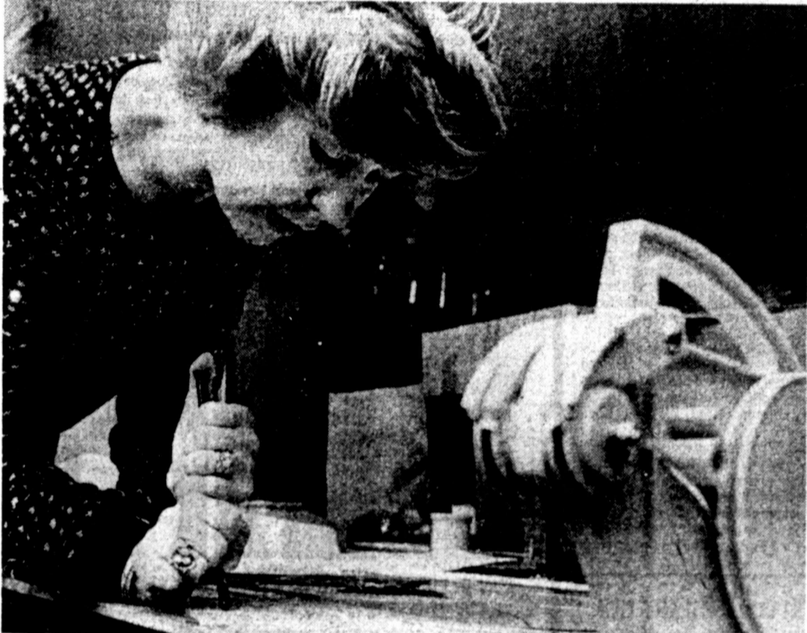
CUTTING THE GLASS — Diana Pool demonstrates the ease of cutting stained glass. With just a little pressure from the thumb of her left hand, she cuts following the lines marked with a felt-tip marker. (Staff Photos by Wayne Wallace)
