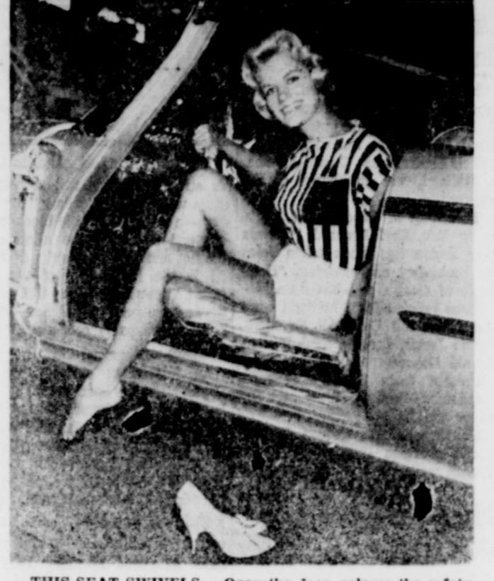
THIS SEAT SWIVELS—Open the door, release the safety-latch, and the seat swings out automatically on this 1960 Dodge. Reverse the body english and the seat swings back and locks in normal driving position. The girl: Judy Bernd of Los Angeles.
