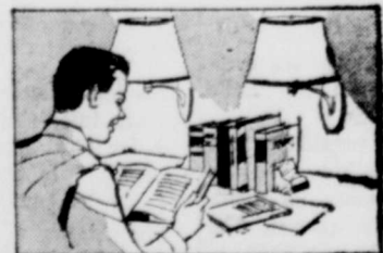
Two wall lamps with 100-watt bulbs in diffusing bowls may be used when study table is placed against a light-colored wall.
