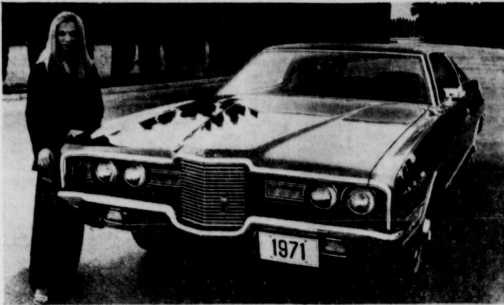
The 1971 Ford LTD is highlighted by this new front end treatment featuring a forward-thrusting center grille section and dual exposed headlamps. This LTD two-door Brougham includes a new, standard high back bench seat which eliminates the need for separate headrests. Ford's new side impact protection system, flush door handles, concealed windshield wipers and a new two-tiered, coved instrument panel also are standard features of the 1971 Ford.
