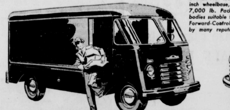
FORWARD-CONTROL CHASSIS Model 3942—137-inch wheelbase, Maximum G.V.W. 10,000 lb. Also available in model 3742—125 1/4-inch wheelbase, Maximum G.V.W. 7,000 lb. Package Delivery type bodies suitable for mounting on the Forward-Control Chassis are supplied by many reputable manufacturers.
