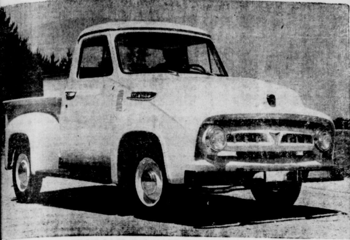
Available with fully automatic Fordomatic transmission for the first time, this new 1953 Ford F-100 series of pick-up and panel delivery trucks meets nearly 50 percent of all hauling needs. It also is available with four other transmissions including automatic overdrive. The F-100 features an entirely new "driverized" cab termed "the roomiest, most comfortable truck cab on the road"; a new one-piece, curved windshield and a 4-foot wide rear window.
