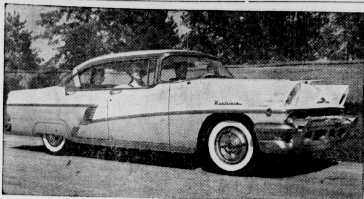
Mercury's newest model—the Montclair Phaeton—features extra eye-level visibility for rear seat passengers and unequalled ease of entrance and exit. It is a low-silhouette, four-door pillarless hardtop only 58 3/4 inches high and more than 17 feet long. The new Phaeton is powered by Mercury's safety-surge V-8 engine with 225 horsepower and a 9.0 to 1 compression ratio. A 210 horsepower V-8 engine also is available with standard transmission. Like all 1956 Mercurys, the new model has a safety steering wheel and five other "crash-tested" safety features.
