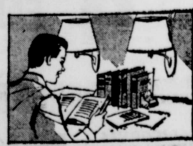
Two wall lamps with 100-watt bulbs in diffusing bowls may be used when study table is placed against a light-colored wall.
