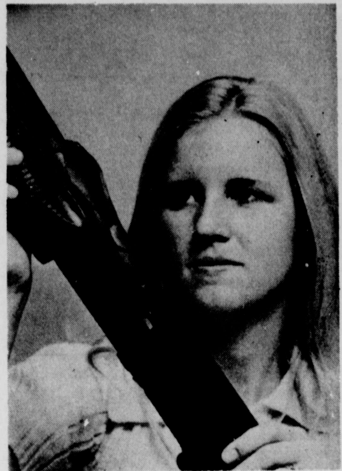
SHOTGUN BURST —Shannon Miller of the Texas Parks and Wildlife Department's Hunter Safety staff shows what happens when a careless hunter uses 20-gauge shotgun shells in a 12-gauge gun. During 1974, 110 Texans were involved in hunting accidents and 16 lost their lives. The Texas Parks and Wildlife Department administers a Volunteer Hunter Safety Program which is open to everyone 12 years of age or older for a $1 registration fee. Department officials say that now when hunting season is over is the time to enroll in a hunter safety class. Local game wardens maintain lists of instructors. TP&WD photo.
